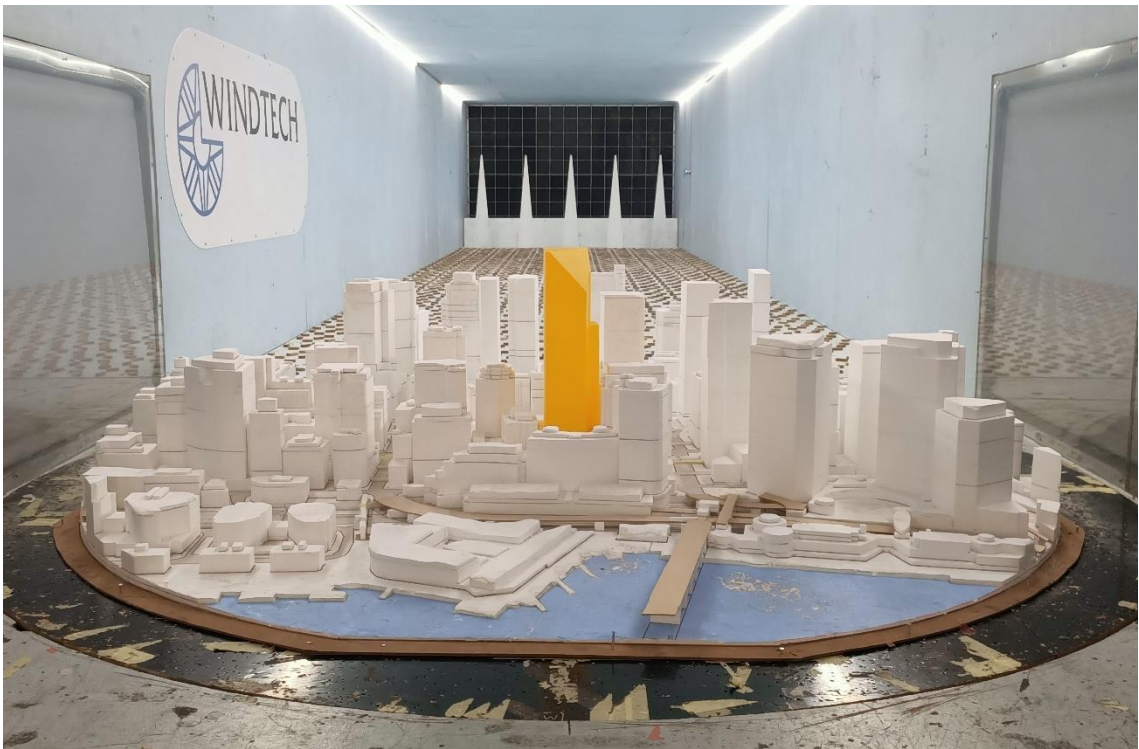
Figure 2c: Photograph of the Wind Tunnel Model Envelope Case, view from the west
